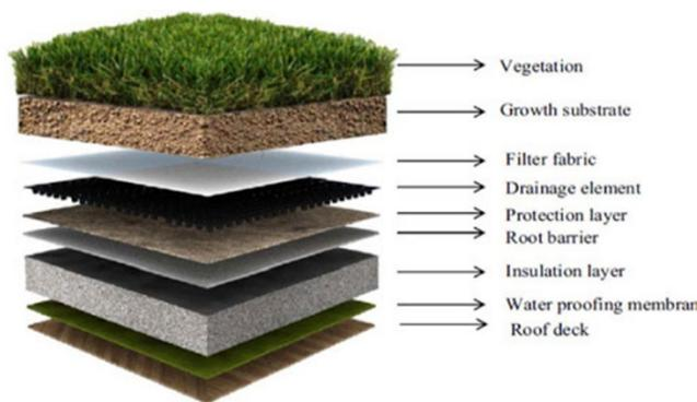
very complex with their structure that varies with the kind of green roof that is built. One of the disadvantages to green roofs is that they are heavy which can set drawbacks to older buildings. Green roofs are heavy in nature because they need many layers to support the vegetation and protect water damage to building's roof tops (Vijayaraghayavan, 2016, p. 744).
