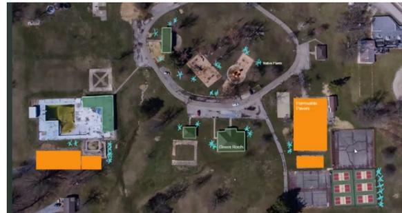
Permeable pavers are the ideal solution, but permeable poured concrete is a good alternative if more cost-effective. **Permeable pavers or permeable poured concrete should be used in the highlighted orange areas at the city park.** These are parking lot areas that take up a lot of space.
